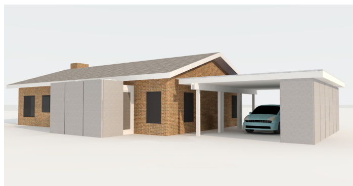
Figure 6. View of REEMs attached as saddlebags to a typical ranch house without obstructing the existing roofline.
